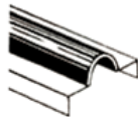
CURB FLANGE For factory manufactured curb systems or field installed wood curbs
