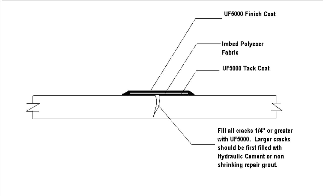
When addressing transitions from floor to wall, the procedure for preparing the joints and coating with ULTRA-FLEX 5000 using a reinforcing fabric is shown below.
