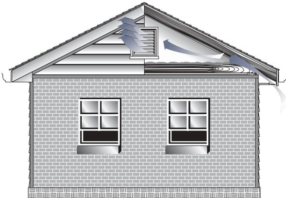
A gable louver, an exhaust vent, allows unwanted air to flow out of the attic. These are located at the ends of the attic.
