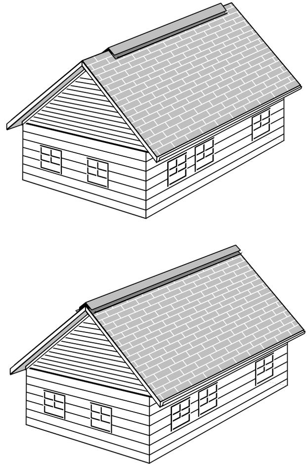
(Top) Ridge vent installed shorter than the ridge length presents an awkward “broken” appearance.
