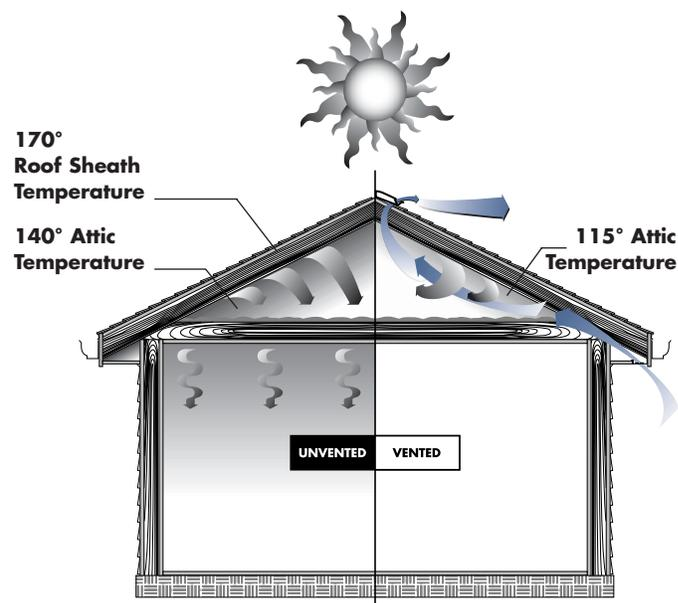
Unvented: Radiant heat penetrating through roof sheath and attic enters living areas of home.
