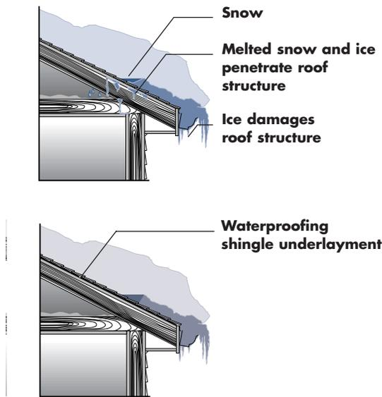
(Top) Water can penetrate to an unprotected roof sheath causing the roof sheath to rot.
