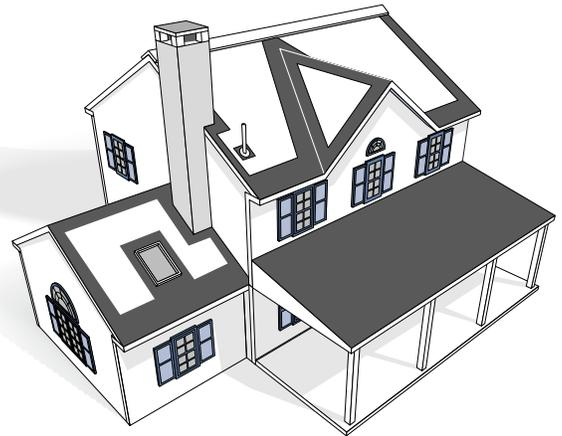
The dark shaded areas are the places that waterproofing shingle underlayment helps protect from the melting water coming off the ice dam.
