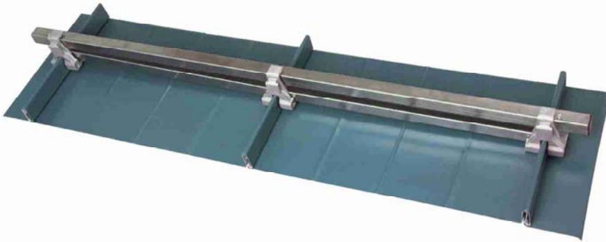
After Castings are installed, fit the square tubing rails into the receiver pockets. For the rail in the lowest position of the standing seam, rail must be cut to the width of the metal roof panel seams. A dab of Surebond Everseal (SB-190), or Surebond Everflex (SB-1800)\* may be used in the receiver pockets to ensure a snug fit.
