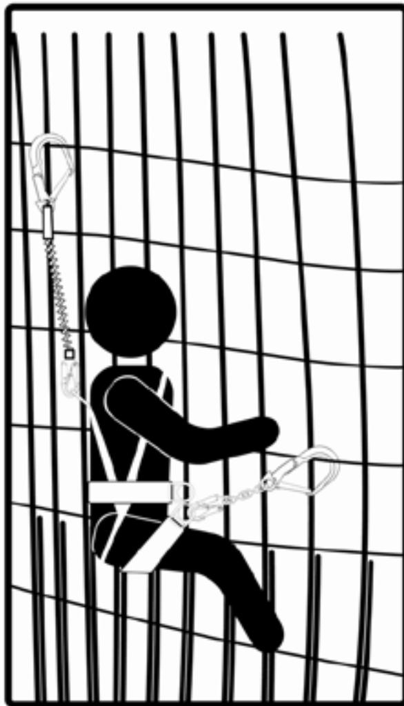
**WARNING:** Side/hip and seat sling D-rings must never be used for any purpose other than work positioning, and no connections of any kind should ever be made to a side or hip D-ring, except for work positioning. **NEVER** attach a Shock-Absorbing Lanyard or Self-Retracting Lifeline to side/hip or seat sling D-rings. **NEVER** use side/hip and seat sling D-rings as a lanyard keeper. **Misuse of these D-rings may result in serious bodily injury or death.**
