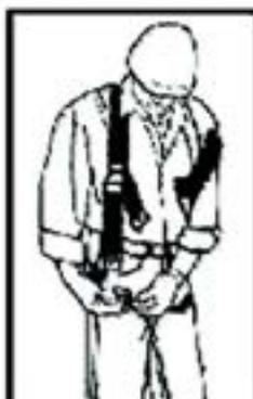
3C: Buckle the leg straps and adjust so that they are snug, not tight. (see FIG. 3.2)
