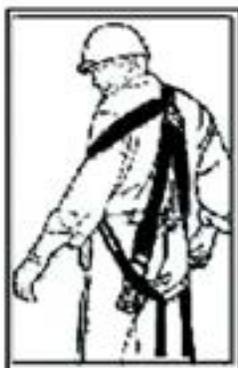
3B: Put on the Harness, so that the back D-ring is in the back between your Shoulder blades.
