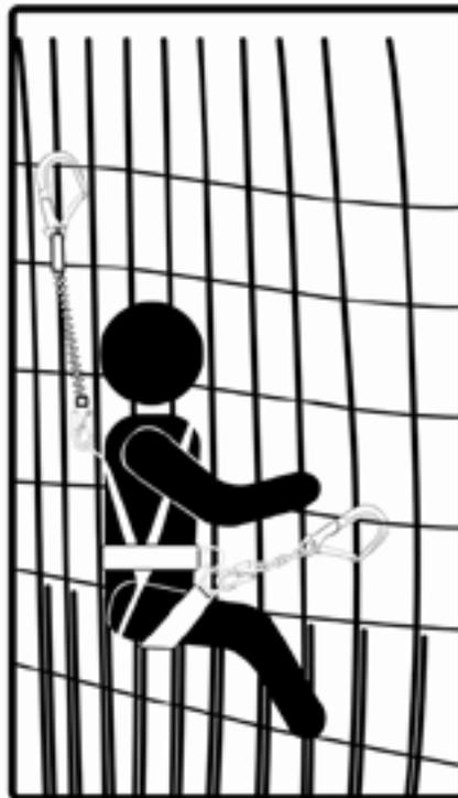
**Warning:** Never attempt to attach any Shock-Absorbing Lanyard, Restraint Lanyard or Self-Retracting Lifeline to either the hip or side D-rings on the waist pad or to the D-rings on the seat sling of this product. Any attempt to utilize these connection points for any purpose other than work positioning (as described in section 3.7 of this manual) **MAY RESULT IN SERIOUS INJURY OR DEATH.**
