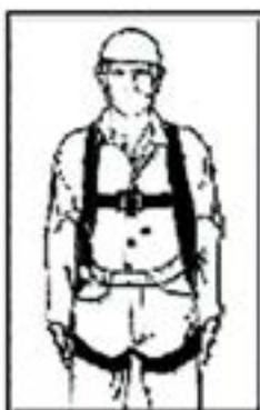
3F: Back D-ring centered between shoulder blades. Chest strap nipple to nipple and sub-pelvic strap below the buttocks.
