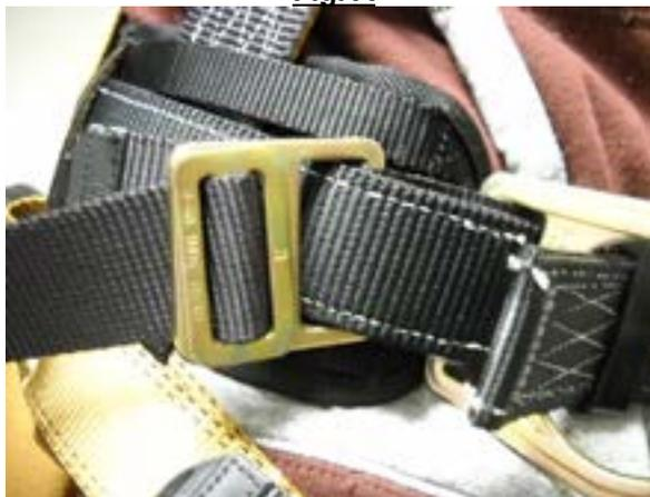
3. Once the sling is installed, adjust the straps to provide better lower back support while working hands-free. When properly adjusted, you should feel about a 50/50 distribution of support between the lower back and the seat. To check your adjustment, use a positioning device in a safe location where you will not be exposed to a fall hazard.
