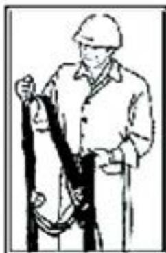
3A: Hold Harness by the back D-ring and allow uncuckled straps to fall free.
