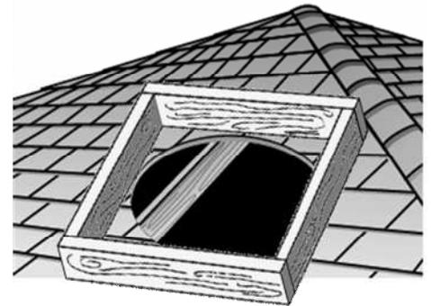
Fig. 2 - Mounting the Curb Box
