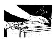
**9.** If band needs additional tightening, pull long handle back from position "A" to position "B". Tighten band with short easy strokes from or "B" to "C"
