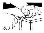
**5.** Pull the band tightly around the box and through the buckle. Note one inch distance between buckle and box edge, also correct position of underlap.
