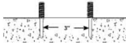
Setting fasteners too close together in concrete or masonry can cause cracking. The recommended minimum distance between fasteners is 3" center to center.
