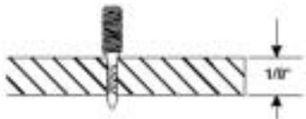
Steel base materials should be a minimum of 1/8" in thickness.
