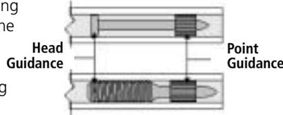
guidance for the fastener. Generally, head guidance is provided by the diameter of the fastener head or threads. 1/4"-20 threaded studs also have a plastic cap to protect the threads of the fastener during the driving process providing head guidance.
