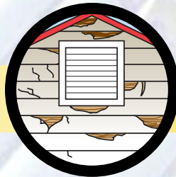
Moisture and uneven temperatures causing peeling of outside paint and wood surfacing
