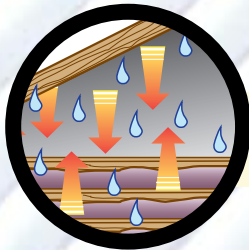
Year round energy waste from attic heat build-up and moisture-laden insulation
