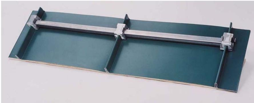
After installing the castings, fit the square tubing rails into the receiver pockets. For the rail in the lowest position of the standing seam, rail must be cut to the width of the metal roof panel seams. A dab of Surebond Everseal (SB-190), or Surebond Everflex (SB-1800)\* may be used in the receiver pockets to ensure a snug fit.
