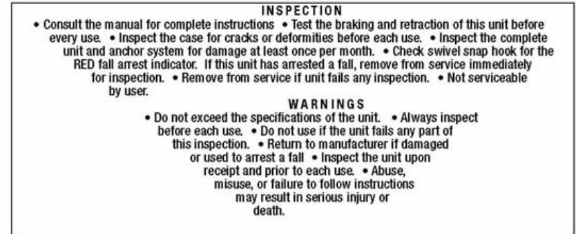
Warning label for FallTech Web SRL's 7270WR, 7271WR and 7270KV (Located on rear housing)
